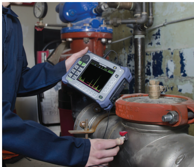
Fig. 1 — A technician performs ultrasonic testing on a welded pipe. (Credit: Olympus Scientific Solutions of America.)
